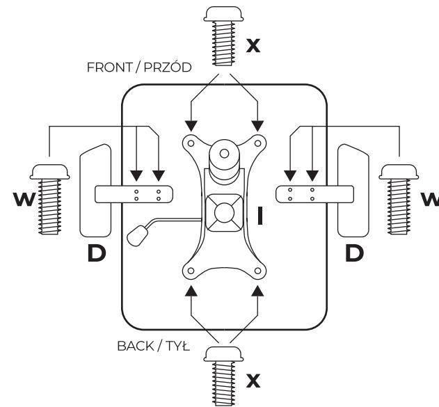
**EN:** Using M8x20mm screws **(x)**, assemble the mechanism **(I)** to the seat as shown. Then assemble the armrests **(D)** to the seat using M8x25mm screws **(w)**.
