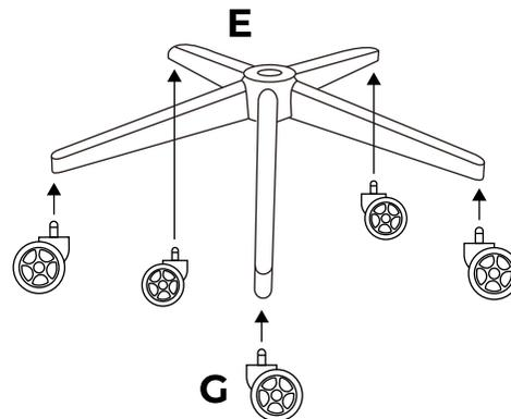
**EN:** Insert the casters (G) into the base (E) using force.
