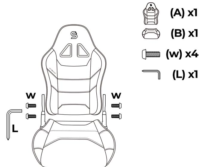
**EN:** Assemble the backrest (A) to the seat (B) using M8x30mm screws (w) and hexagon key wrench (L).
