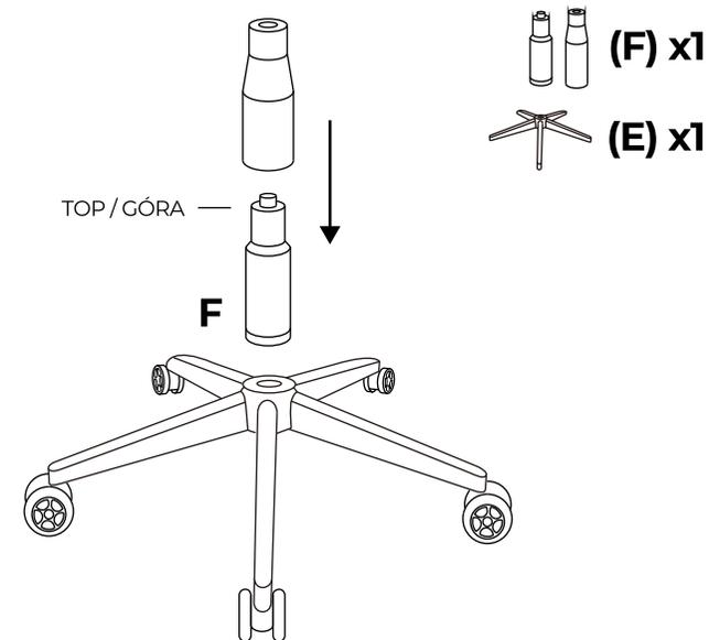
**EN:** Place the gas lift (F) in the middle of the base (E) and put the plastic cover on it.
