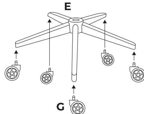
**EN:** Insert the casters (G) into the base (E) using force.
