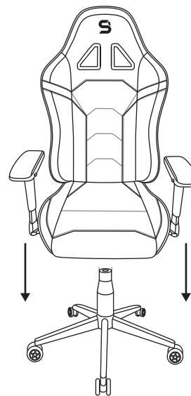
**EN:** Insert top of the gas lift into to the mounting hole of the mechanism under the seat (you may need help of another person). Push the seat down firmly.
