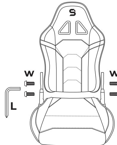
**EN:** Assemble the backrest (A) to the seat (B) using M8x30mm screws (W) and hexagon key wrench (L).
