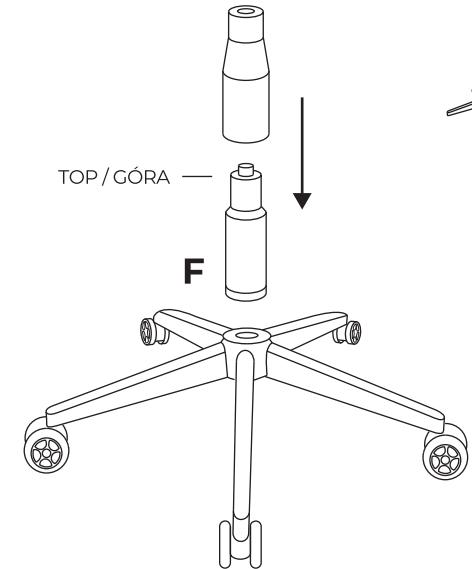
**EN:** Place the gas lift (F) in the middle of the base (E) and put the plastic cover on it.
